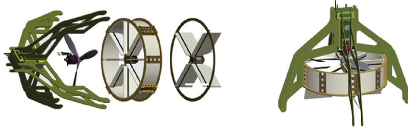
Fig. 5. The prototype of miniature ducted-fan aerial vehicle described in [28].
